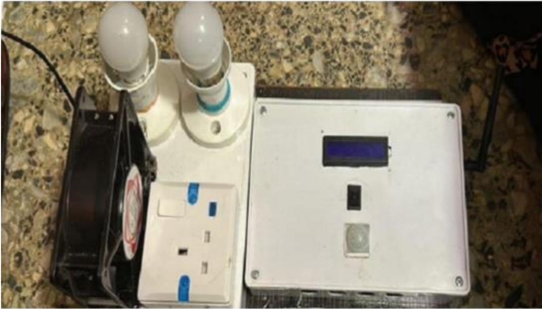
Figure 10: Prototype of the Home Automation System in OFF State
